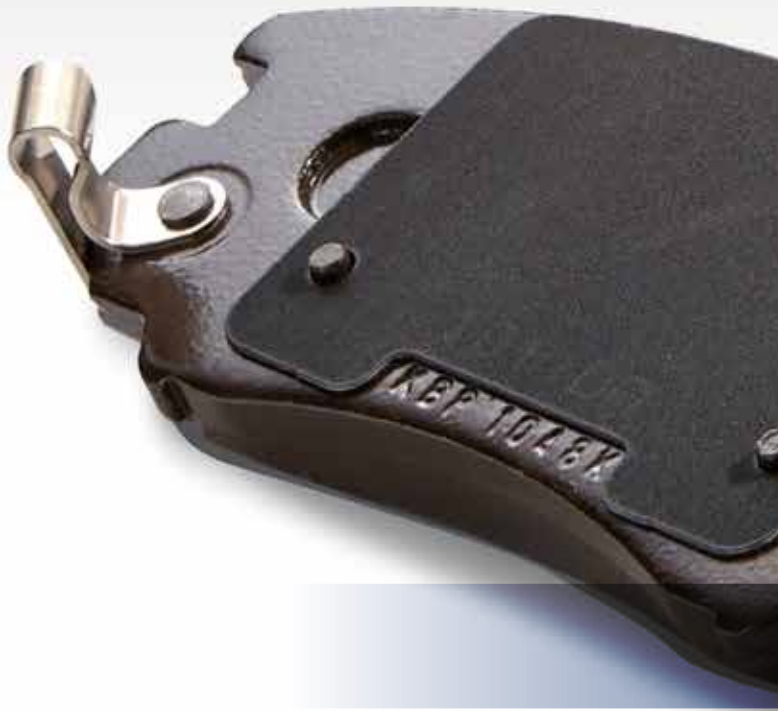
Figure 1. Genuine brake pad is rather compressed in size but heavy, showing smoother cuttings with well-defined colors inside
